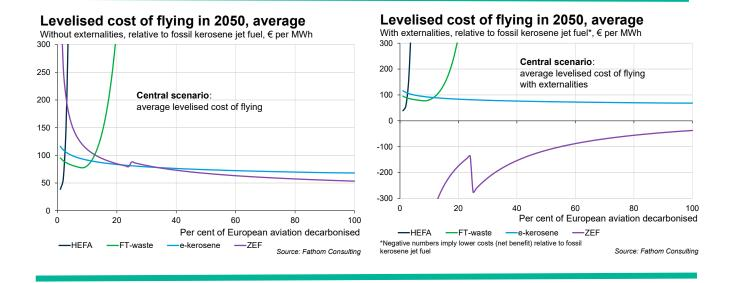
To support our research we built <u>Fathom's Aviation Decarbonisation Model, FADM</u>, which shows the how the levelised costs of different decarbonisation technologies vary relative to fossil kerosene under different scenarios, at different points in time and at different levels of decarbonisation; it can also be used to assess the costs and benefits from the perspective of both the aviation sector and the wider economy through considering externalities
